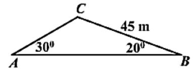
Para hallar b procedemos en forma similar  $\frac{45\text{m}}{\text{sen}30^\circ} = \frac{b}{\text{sen}20^\circ}$   $\frac{45\text{m} \cdot \text{sen}20^\circ}{\text{sen}30^\circ} = b \rightarrow b = 30.78 \text{ m}$
